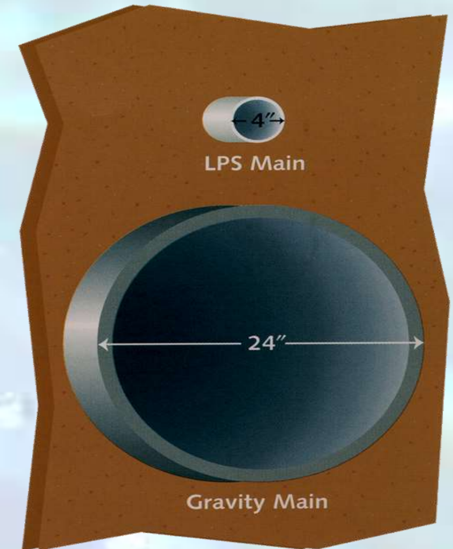
Smaller diameter piping. E/ONE low pressure sewer systems require vastly smaller-diameter piping: 4 inches instead of gravity's typical 24 inches.
